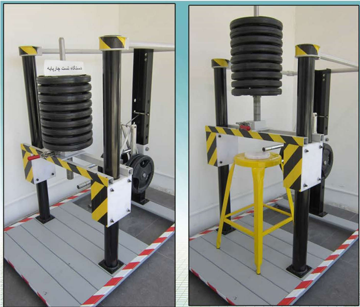
Mechanical testing device (for testing the strength and stability of products)
